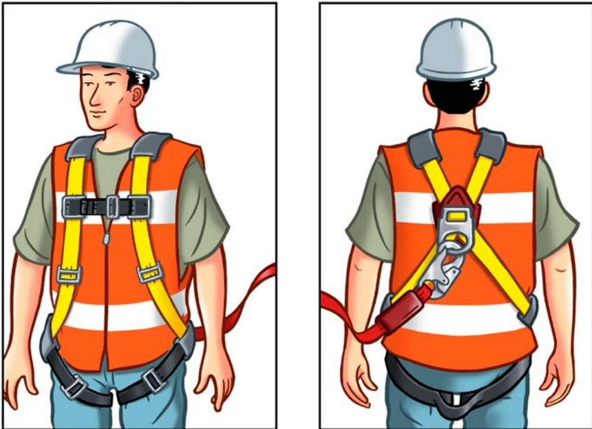
Harness and Fall Arrest Shock Absorbent Lanyard/Lifeline
